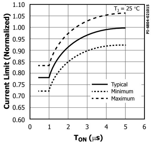
Figure 22. Current Limit vs.  $T_{ON}$  for TNY288~290.
