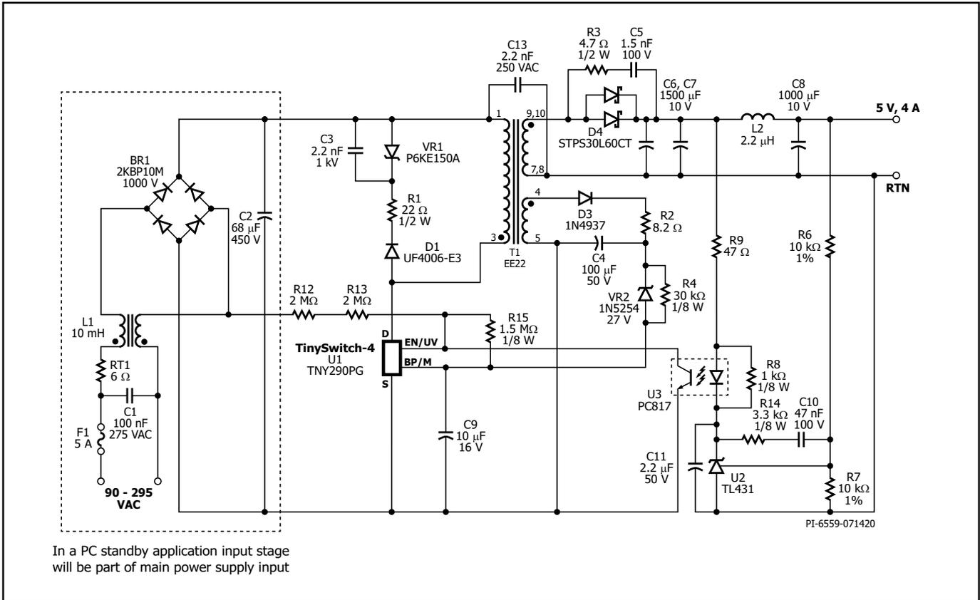
Figure 16. TNY290PG, 5 V, 4 A Universal Input Power Supply.
