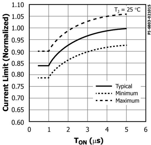
Figure 21. Current Limit vs.  $T_{ON}$  for TNY284~287.
