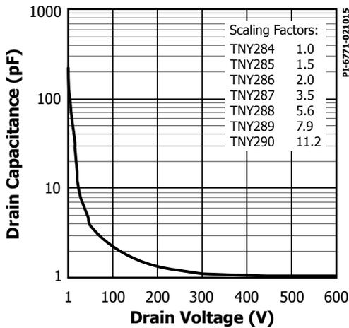
Figure 27. C<sub>oss</sub> vs. Drain Voltage.
