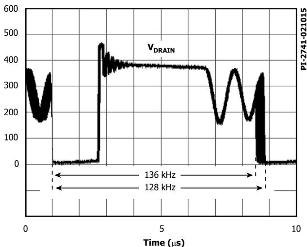
Figure 5. Frequency Jitter.
