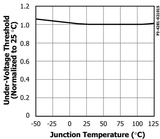
Figure 29. Undervoltage Threshold vs. Temperature.
